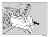
Remove the red sheet from the PCU, and then remove the two strips of tape.
